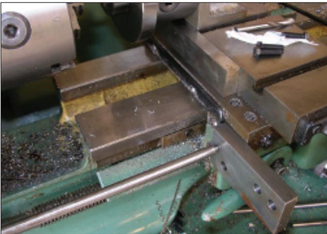
**Photo 8.** Setting the stop so the drill can't go too deep.
